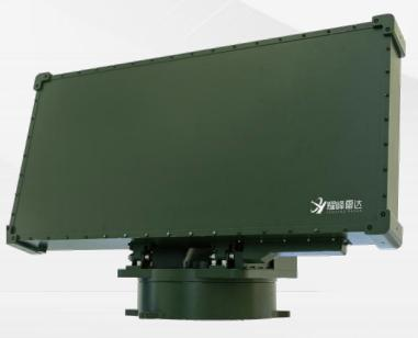
YFR-13 three-coordinate radar of pulsed Doppler system with azimuth sweep + pitch phase sweep system can detect and locate lowaltitude flying objects (unmanned aerial vehicles and birds), which is mainly used in the field of bird sentiment prevention and control in airports.
