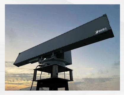
YFR-12 is a pulse Doppler system radar that can detect and locate the UAV and surface ships at the same time, mainly used for the safety protection of the coastline.
